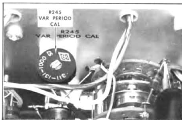
Fig. 5-24. Location of period timing adjustment on bottom side of Type 115 chassis subpanel.
